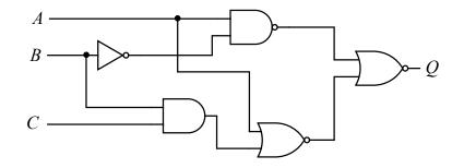
Your task is to design a simpler circuit that will produce the same truth table. You should do this by first writing down a logic expression that represents Q in terms of A, B, and C. Then simplify your expression using some of the identities and theorems that you proved in problem 2. This circuit can be replaced with two gates! Note that wires that intersect without a dot are *not* connected.
